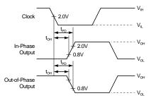
Figure 11. Voltage Waveforms - Propagation Delay Times
